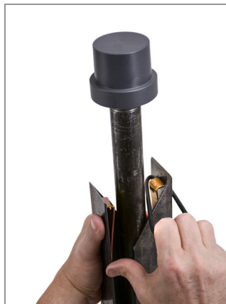
FIGURE 10: Installing the O-Ring
