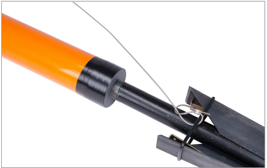
FIGURE 16: Release Cord, made using GEOKON part number 07-062G
