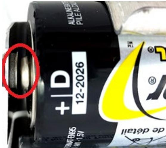
**Faulty Battery Installation**
