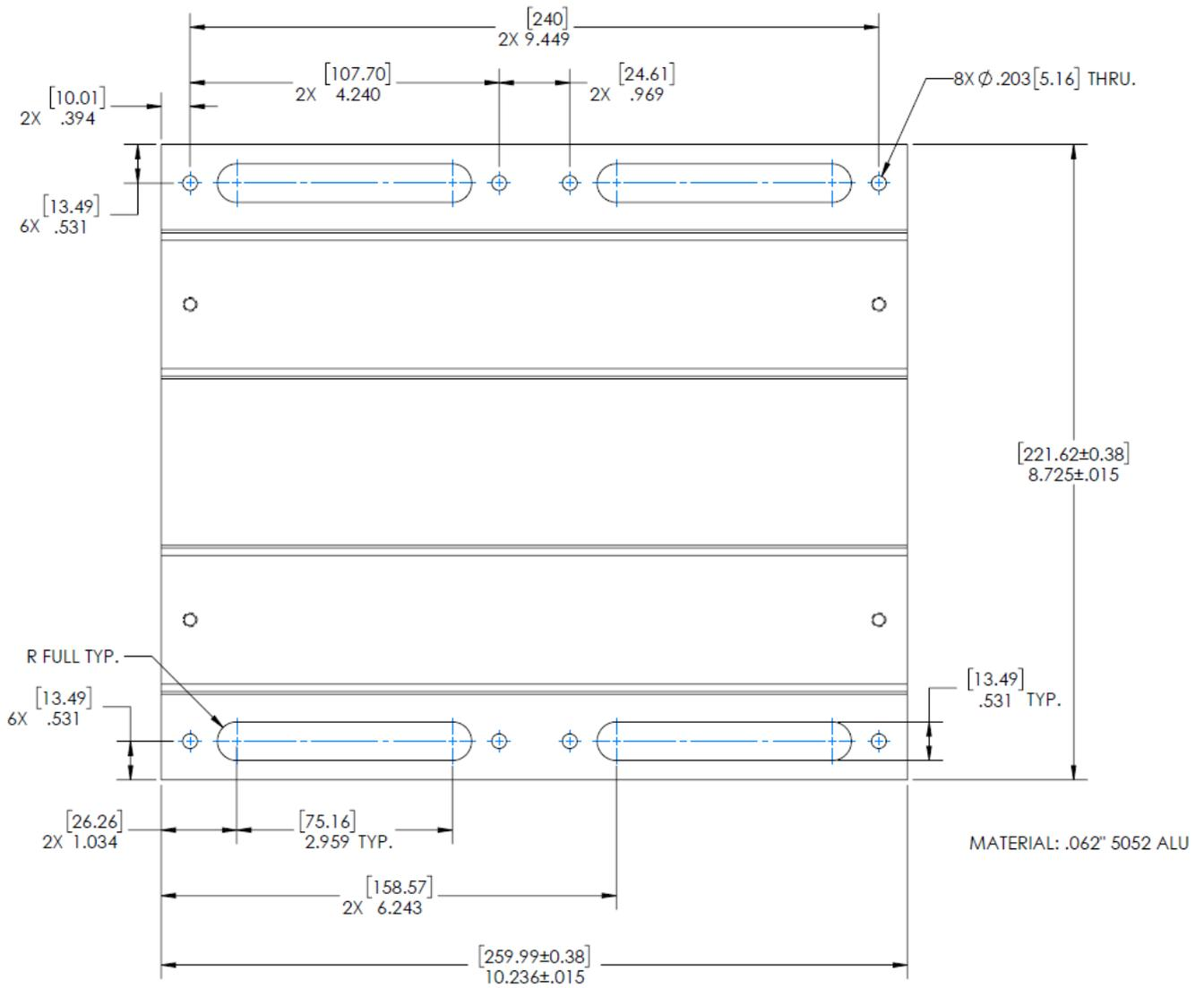
Figure 5 - Model 8002-8 Aluminum Mounting Bracket Dimensions
