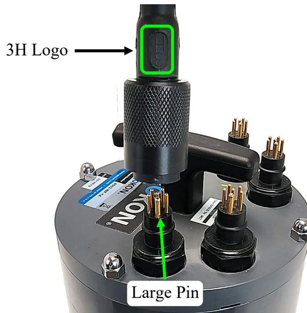
Figure 2 – Connector Alignment
