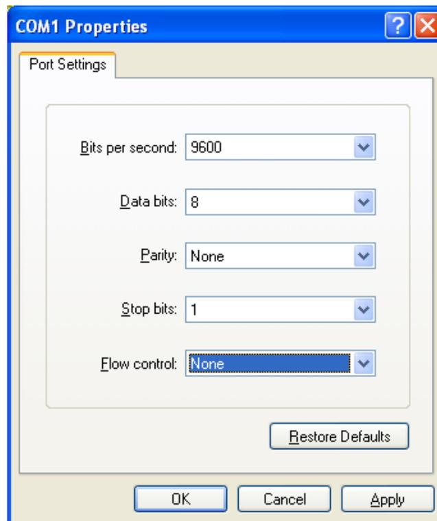
Figure 26 - HyperTerminal COM Port Settings
