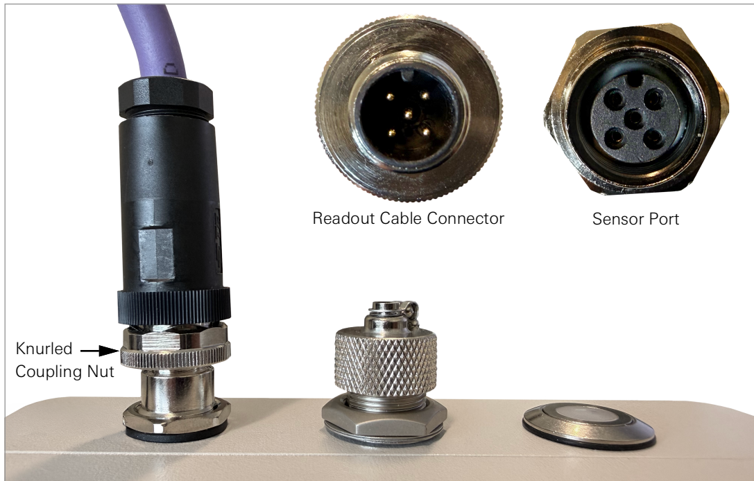
FIGURE 4: Connect the Readout Cable to the StringLink
