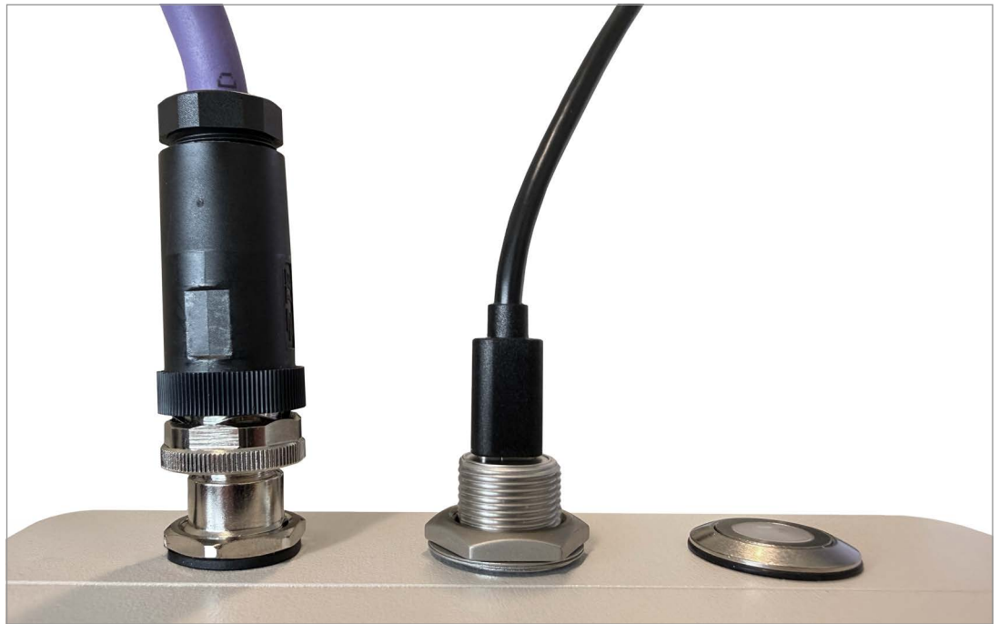
FIGURE 5: Connect the USB Cable to the StringLink
