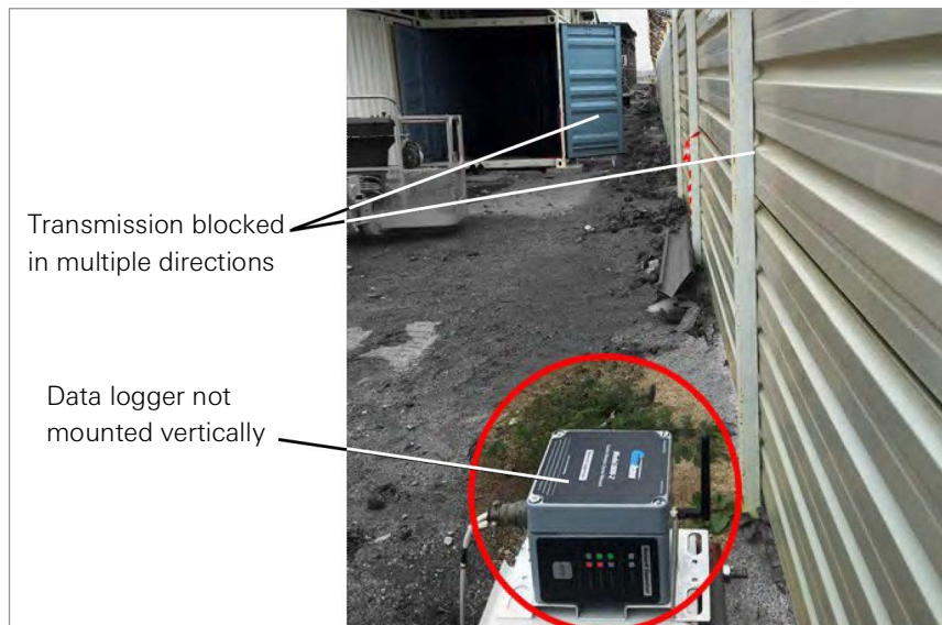
FIGURE 19: Installing Close to Buildings or Fences/Walls, and/or Horizontally
