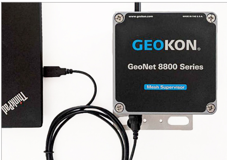
FIGURE 47: USB Cable Connection (COM-166 Pictured)
