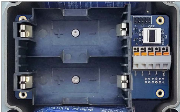
FIGURE 73: PCB Aligned with Standoffs
