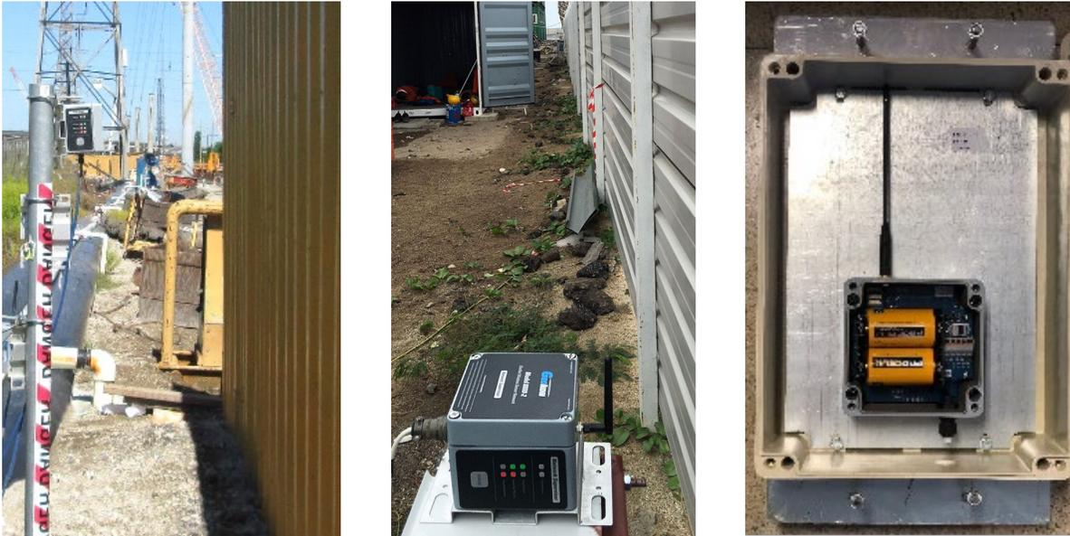
Figure 3 - Examples of Radio Obstructions
