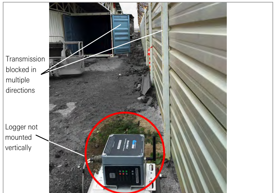
FIGURE 18: Installing Close to Buildings or Fences/Walls, and/or Horizontally
