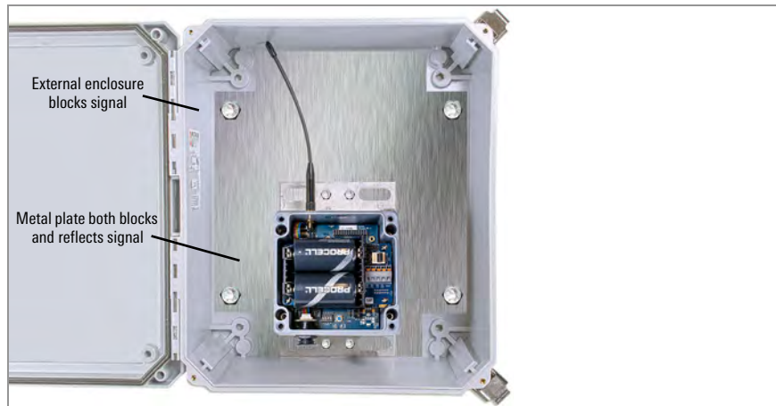
FIGURE 19: Mounting onto a Metal Plate and/or Inside an Enclosure
