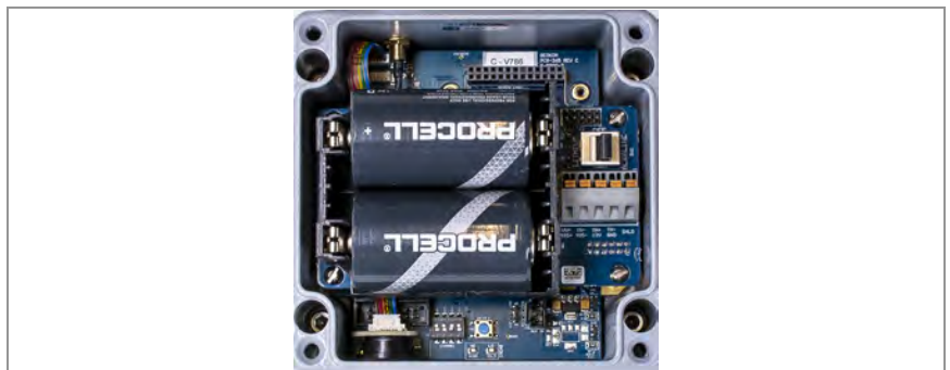
FIGURE 16: Battery Switch Location Detail
