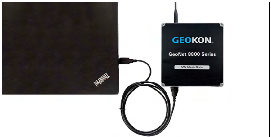
FIGURE 36: USB Cable Connection
