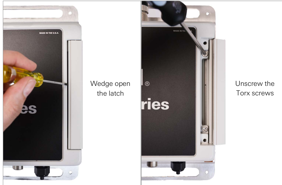
FIGURE 8: Open the Cover of a DHP Data Logger
