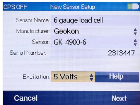
**FIGURE 5:** Enter Applicable Sensor Information (6 Gauge Load Cell Example)
