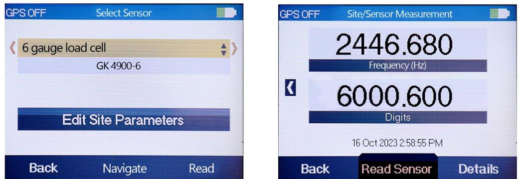
**FIGURE 7:** Site/Sensor Measurement
