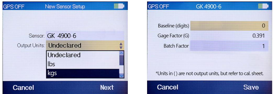
**FIGURE 6:** Enter Sensor Reading Information
