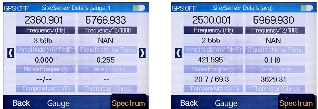
**FIGURE 8:** Individual Gauge Readings (Left, Showing Gauge 1) and Average Reading (Right)
