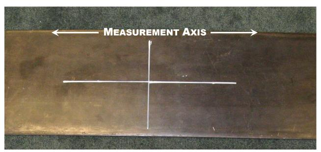
From the transverse mark, make two additional marks at 1.5 inches on either side of the centering mark (see below photo). The areas circled below are the portions of the cross-section that the necessary surface preparations must be performed. Surface preparation techniques are explained in Section 5.2.7.
