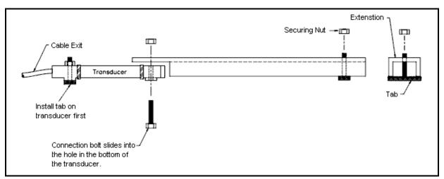
5. There is a machined hole in the non-cabled end of the transducer that will capture a standard <sup>1</sup>/<sub>4</sub> 20 hex head bolt (see picture below). Simply insert the bolt through the bottom of the transducer and twist until the bolt head drops into the hole. There is a relief cut in the back of the extension to accept the protrusion on top of the gage. This will ensure that the gage is positioned correctly.
