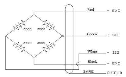
When testing the ST350 Strain Transducer with the intelligent plug the pin out is as follows:
