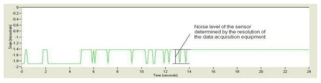
2. Ensure the Strain Transducer returns a smooth output. Run a test at a sample frequency higher than 30 Hz and apply a smooth tension force (gently pulling one each
